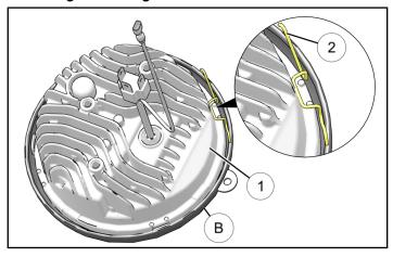
b. Using a small tipped tool (such as a standard screwdriver), press spring clip ② under outer lip of trim ring ®. Ensure center of spring clip stays aligned around metal tabs of LED light housing ①.
