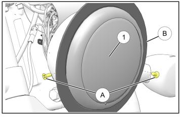
b. Ensure wires for headlight are secured inside the bucket © or wrapped in the harness wrap ①.
